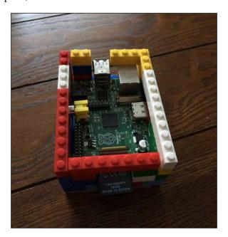
The top of the case does not contain a lid. This is optional and will help to prevent anything from falling onto your Raspberry Pi. However, by not including a lid you can stack cases upon each other, with the base of the top case acting as the lid of the bottom.
